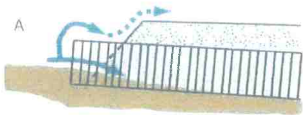
FIGURE 155. Proper culvert installation involves correct culvert orientation, setting the pipe slightly below the bed of the original stream, and backfilling and compacting the fill as it is placed over the culvert. Installing the inlet too low in the stream (A) can lead to culvert plugging, yet if set too high (B) flow can undercut the inlet. If the culvert is placed too high in the fill (C), flow at the outfall will erode the fill. Placed correctly (D), the culvert is set slightly below the original stream grade and protected with armor at the inlet and outlet. Culverts installed in fish-bearing stream channels must be inset into the streambed sufficiently (~25% embedded) to have a natural gravel bottom throughout the culvert (Modified from, MDSL, 1991)
