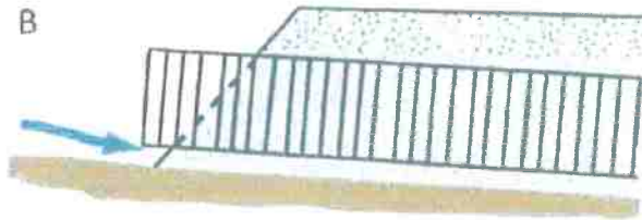
FIGURE 155. Proper culvert installation involves correct culvert orientation, setting the pipe slightly below the bed of the original stream, and backfilling and compacting the fill as it is placed over the culvert. Installing the inlet too low in the stream (A) can lead to culvert plugging, yet if set too high (B) flow can undercut the inlet. If the culvert is placed too high in the fill (C), flow at the outfall will erode the fill. Placed correctly (D), the culvert is set slightly below the original stream grade and protected with armor at the inlet and outlet. Culverts installed in fish-bearing stream channels must be inset into the streambed sufficiently (~25% embedded) to have a natural gravel bottom throughout the culvert (Modified from, MDSL, 1991)
