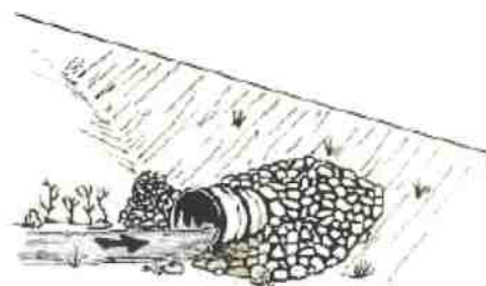
FIGURE 107B. Riprap armor at culvert inlet (Keller and Sheraz, 2003).
