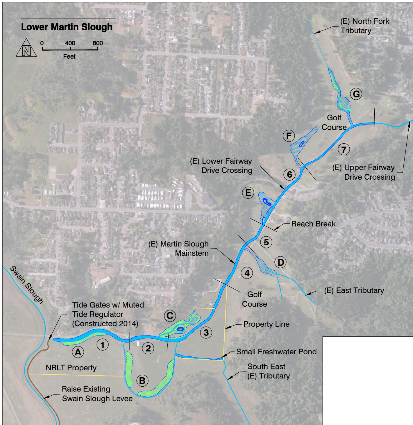
Figure 2-1. Summary of Martin Slough Enhancement Project Components. Reach Number and Pond Name are Circled.
