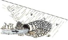
FIGURE 107A. Riprap armor at culvert outlet (Modified from: Kellar et al., 2011).
