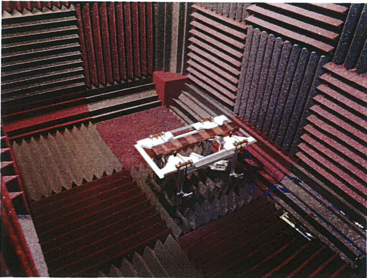
Figure 2-2: Acoustic/modal test stand in anechoo chamber.
