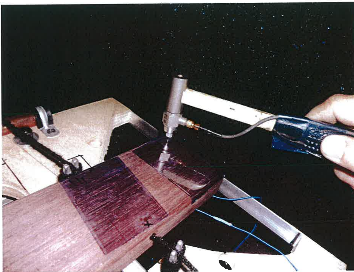
Figure 3-1: Example of a modal impact at location 113Z-.
