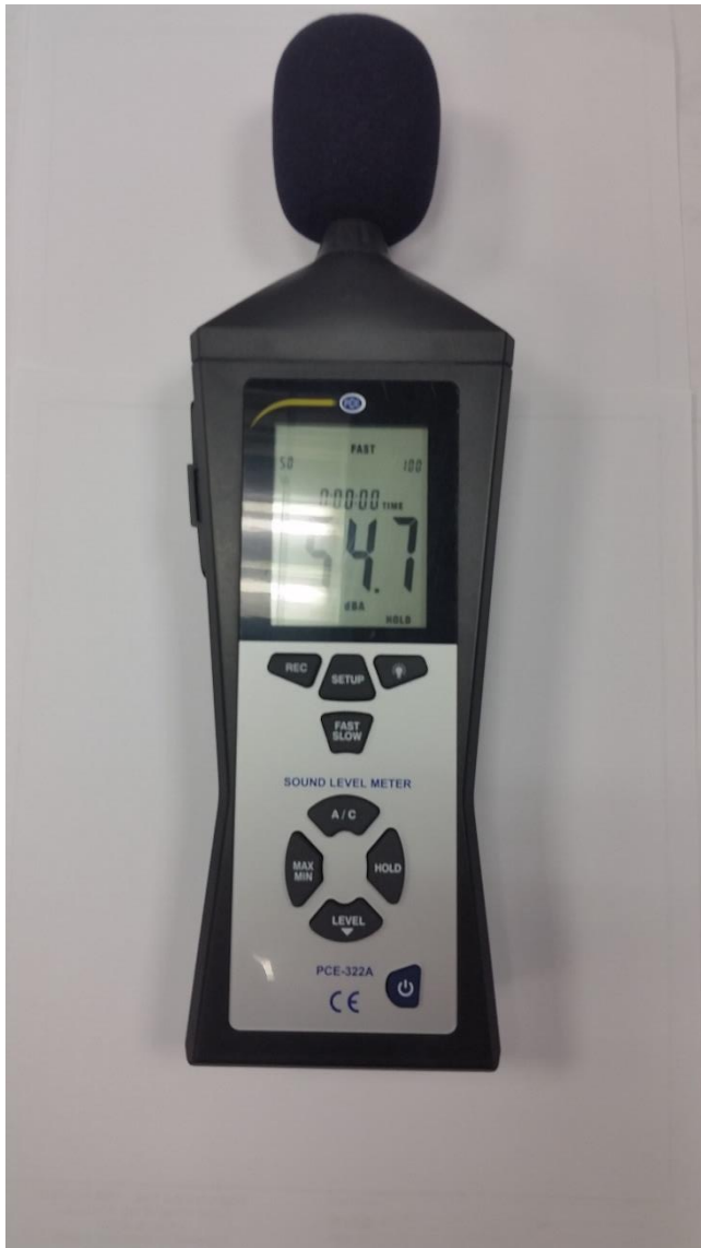
Figure 3: PCE-322A noise meter used in study
