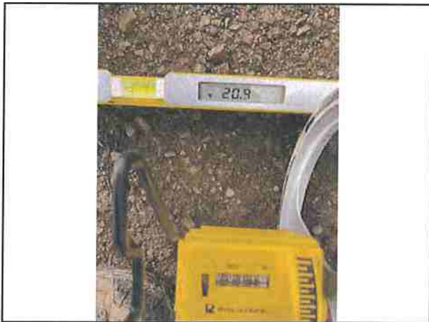
Photo #81 Gorden Rd Slope 20.9% Width 11'6"
