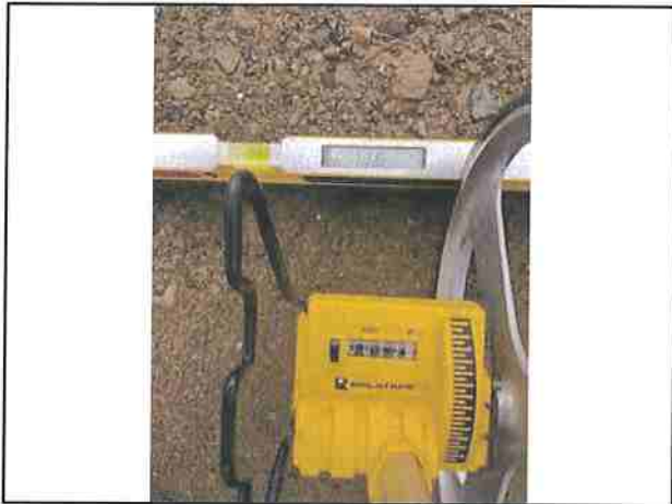
Photo #99 Gorden Rd Slope 13.6% Width 13'2"
