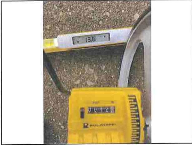
Photo #241 Showers Pass Rd Slope 13.6% Width 12'8"
