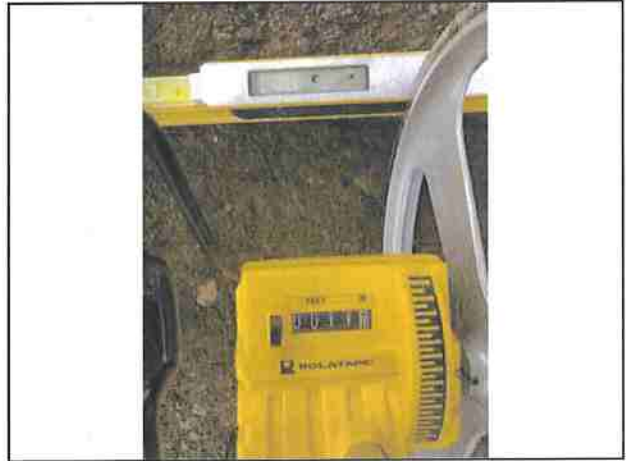
Photo #74 Gorden Rd Slope 13.5% Width 11'0"
