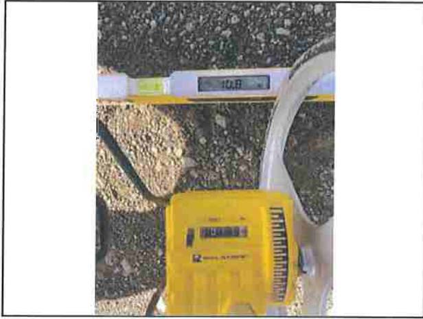
Photo #169 Showers Pass Rd Slope 10.8% Width 11'10"
