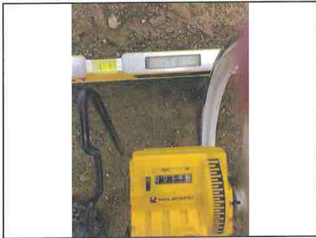
Photo #139 Showers Pass Rd Slope 17.9% Width 14'9"
