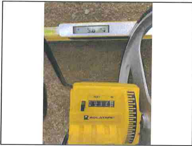
Photo #347 Showers Pass Rd Slope 9.6% Width 12'8"
