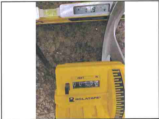
Photo #331 Showers Pass Rd Slope 11.9% Width 15'5"
