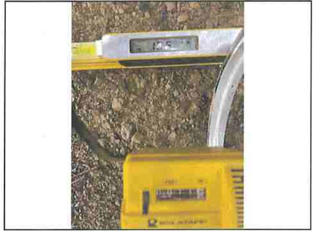
Photo #68 Gorden Rd Slope 19.5% Width 11'8"
