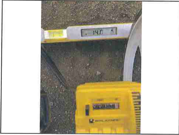
Photo #151 Showers Pass Rd Slope 14.0% Width 14'1"
