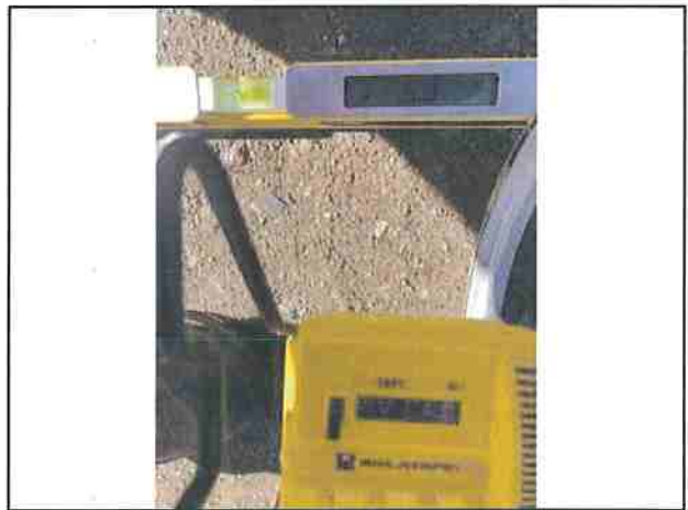
Photo #208 Showers Pass Rd Slope 5.8% Width 12'8"
