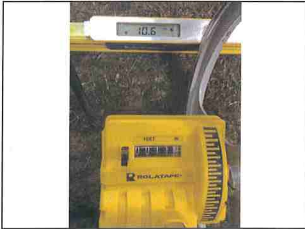
Photo #19 Private Access Rd APN APN 317-023-010 Slope 10.6% Width 11'7"
