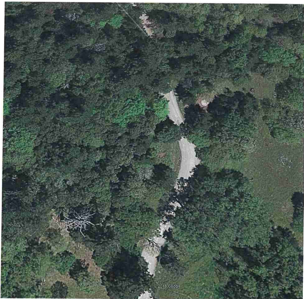
RS5 – The road width at this curve is 20 feet – there is a significant area to pull-out alongside this curve.
