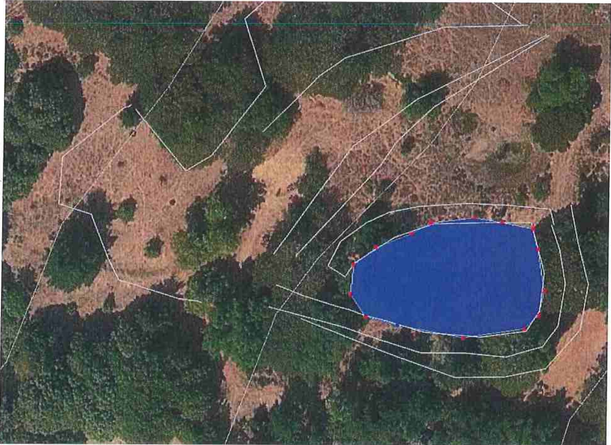
Figure 8: Aerial Image dated 8/24/2012 which shows the native ground configuration upstream of the pond. No evidence of channelization noted. Lines correspond to graded areas as shown in the Representative Map, Attachment A
