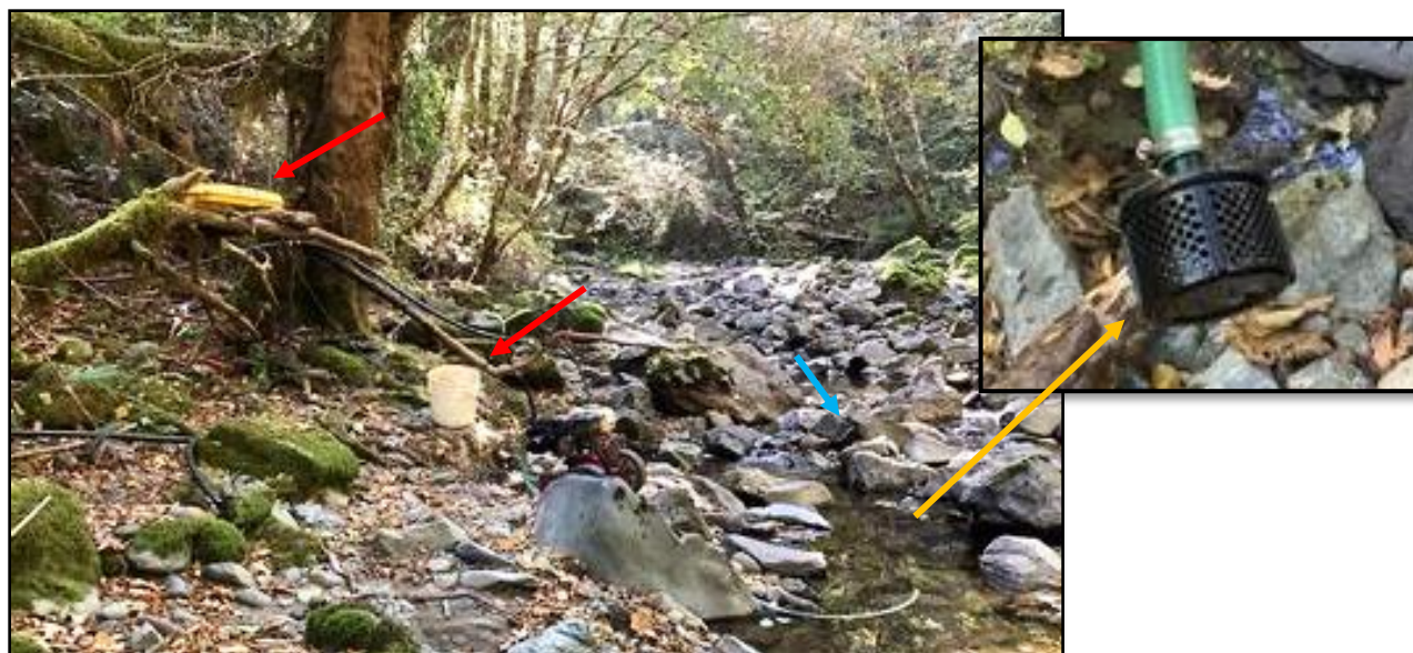
Figure 7. Violation Nos. 3-5 (Map ID WS-1). Looking southeast (upstream) at a gas-pump water diversion located on Little Larabee Creek, a Class I fish bearing stream, during the October 15, 2024, site visit. The intake screen is insufficient to prevent harm to aquatic life. Diverted water was stored on the Property and used for cannabis irrigation. Note the placement of the bucket and gas tank (red arrows). Blue arrow indicates direction of streamflow.
