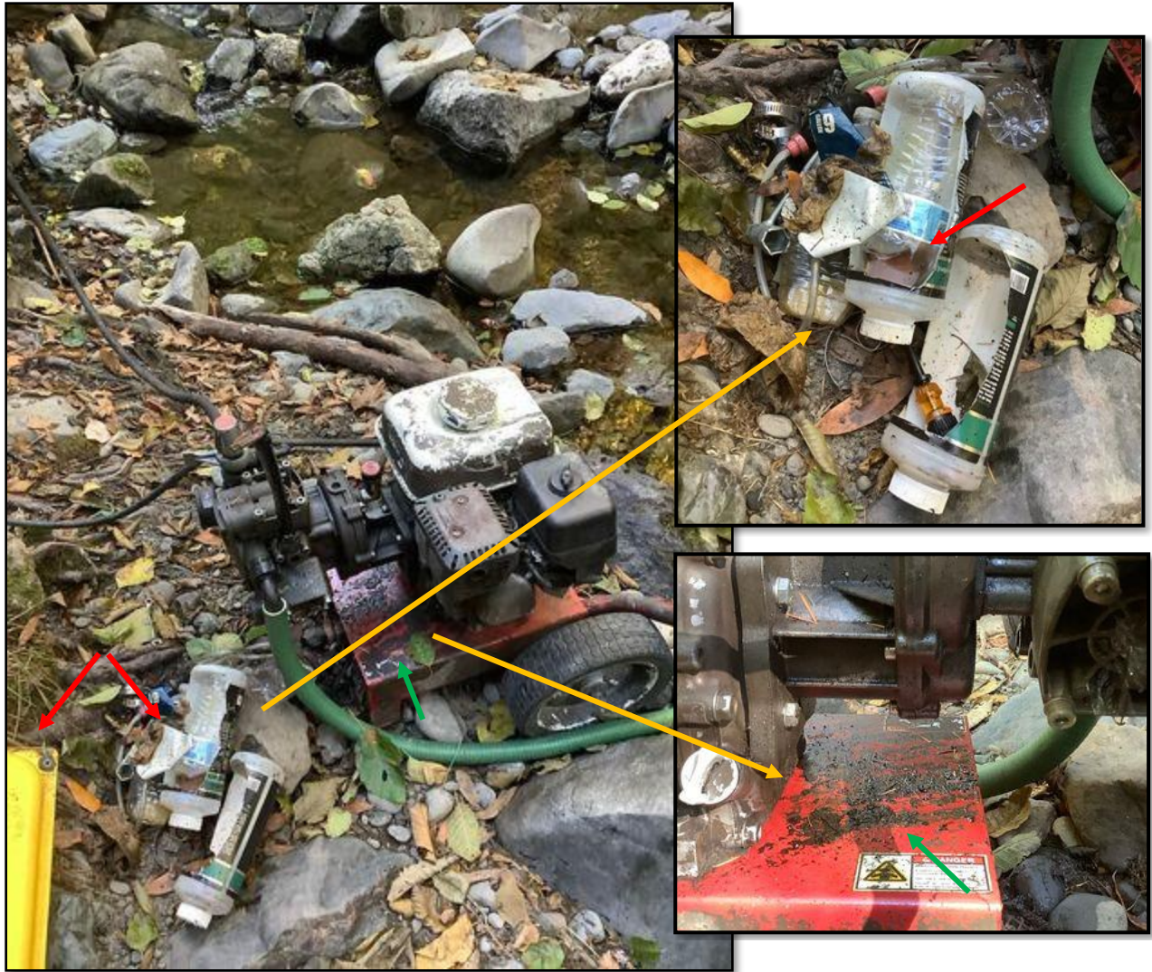
Figure 12. Violation Nos. 3-5 (Map ID WS-1). A close up image of the gas-powered pump and associated fuel and oil containers, used to divert water for cannabis cultivation on the Property. The leaky pump (green arrows) and petroleum products (red arrows) lack proper storage or secondary containment resulting in delivery of petroleum to State waters. Plastic irrigation line, plastic bottles, and other plastic and non-plastic refuse were placed into, and where they could pass into, State waters, resulting in water pollution and potential for future delivery.
