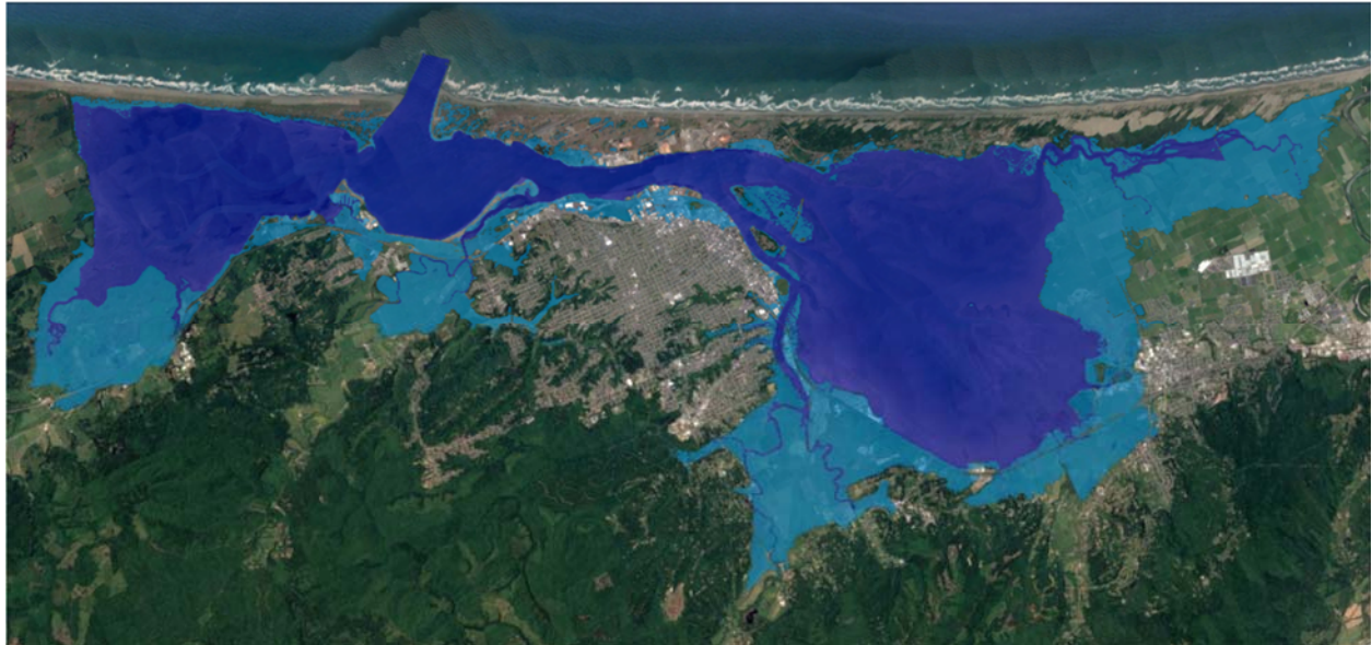
Figure 2. Projected Sea Level Rise Inundation Zone (Stillwater) on Humboldt Bay for Mean Monthly Maximum Tide with 3.3 feet (1.0 meters) of Sea Level Rise.
