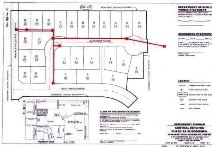
Above: Diagram showing the storm drain system to be maintained by the county as part of the proposed division for road maintenance.
