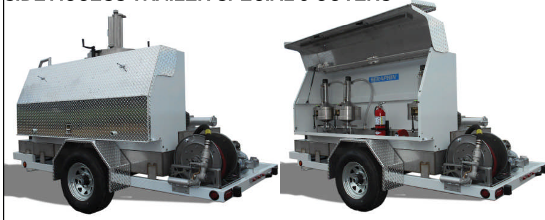
TOP PANEL AND BOTTOM PANEL FOLD UP ASSISTED BY GAS SPRINGS
