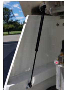
TOP PANEL AND BOTTOM PANEL FOLD UP ASSISTED BY GAS SPRINGS
