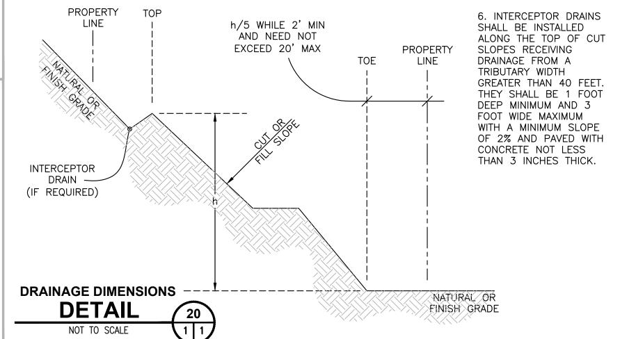
WHERE EXISTING GRADE IS AT A SLOPE STEEPER THAN 5:1 (h:v) AND A DEPTH OF THE FILL EXCEEDS 5 FEET, BENCHING SHALL BE PROVIDED. A KEY SHALL BE PROVIDED THAT IS NOT LESS THAN 10 FEET IN WIDTH AND
