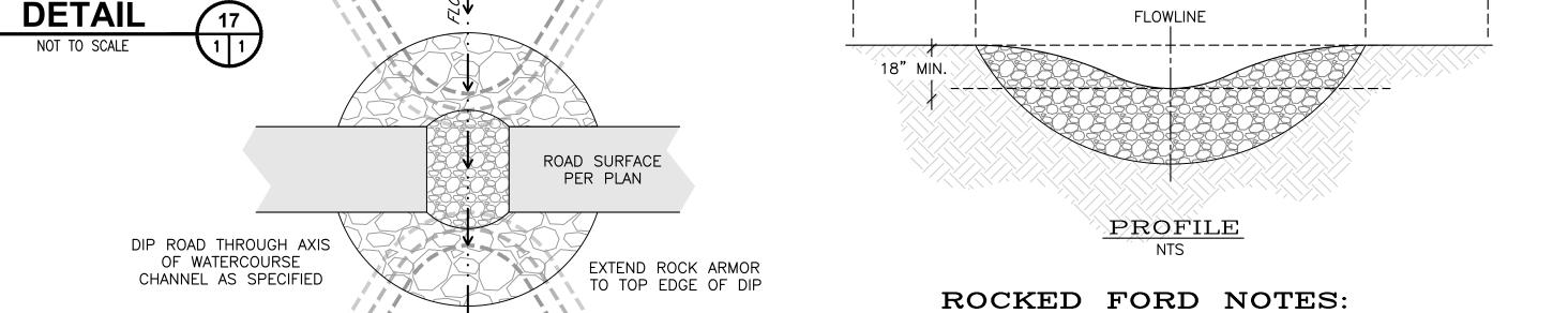
ACROSS ROADS. CHANNEL SPILLWAY 2. THE ROAD SHALL DIP INTO AND OUT OF THE ROCKED FORD TO MINIMIZE DIVERSION POTENTIAL.
