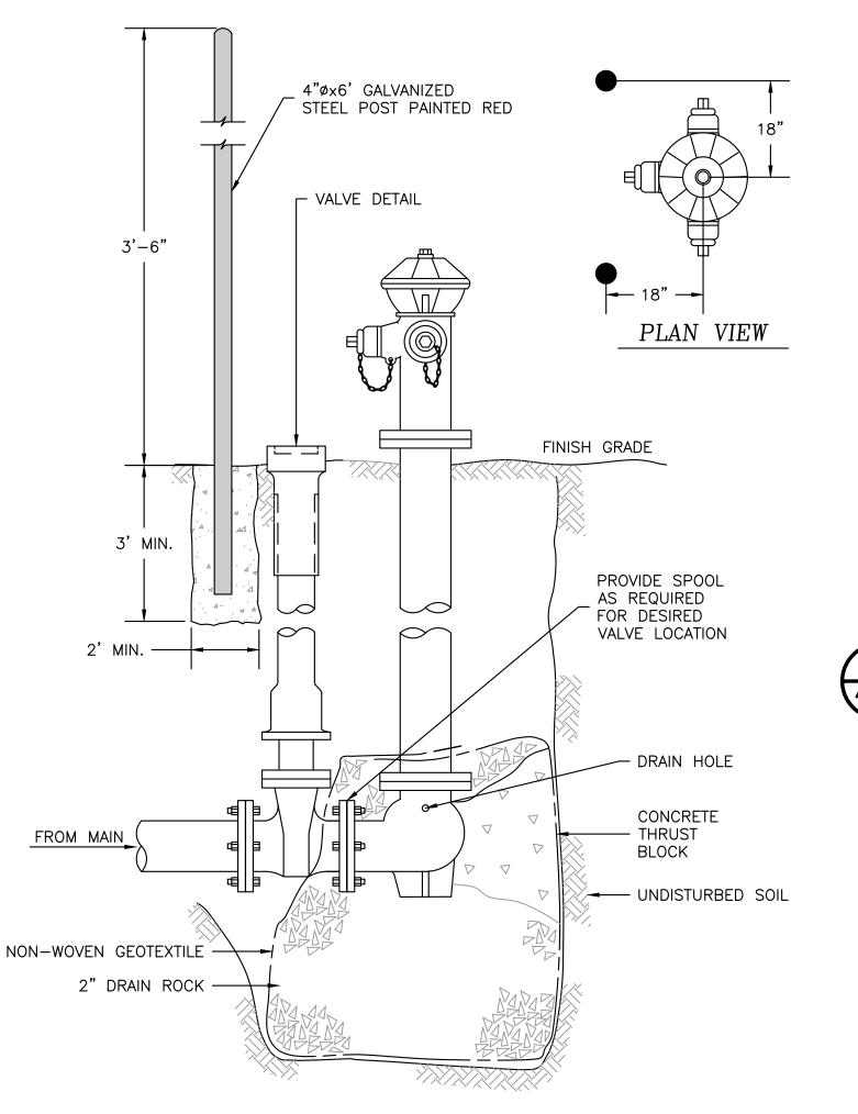
DRY BARREL FIRE HYDRANT DETAIL
