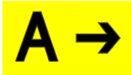
Direction/Runway Exit Sign
