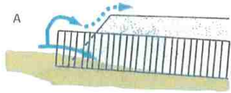
FIGURE 155. Proper culvert installation involves correct culvert orientation, setting the pipe slightly below the bed of the original stream, and backfilling and compacting the fill as it is placed over the culvert. Installing the inlet too low in the stream (A) can lead to culvert plugging, yet if set too high (B) flow can undercut the inlet. If the culvert is placed too high in the fill (C), flow at the outfall will erode the fill. Placed correctly (D), the culvert is set slightly below the original stream grade and protected with armor at the inlet and outlet. Culverts installed in fish-bearing stream channels must be inset into the streambed sufficiently ( \sim 25\% embedded) to have a natural gravel bottom throughout the culvert (Modified from: MDSL, 1991).
