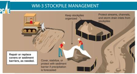
Protection of stockpiles is a year-round requirement addressing wind and water. erosion potential. To properly manage stockpiles:
