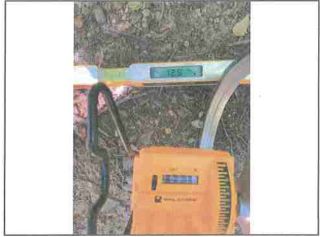
Photo #98 Private Access Rd APN 221-071-020 Slope 12.5% Width 11'3"
