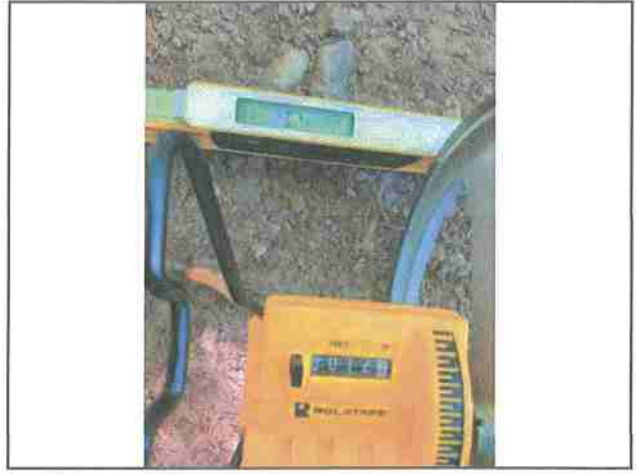
Photo #86 Private Access Rd APN 221-071-020 Slope 23.4% Width 12'1"
