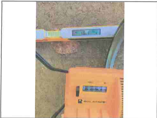
Photo #15 Private Access Rd APN 221-071-020 Slope 16.1% Width 10'8"
