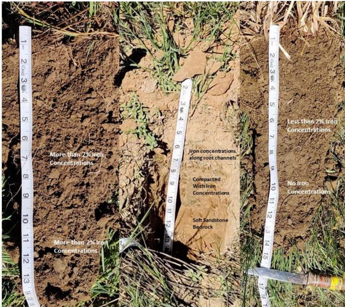
Image 5. Representative soil profiles for non-hydric and hydric soils.
