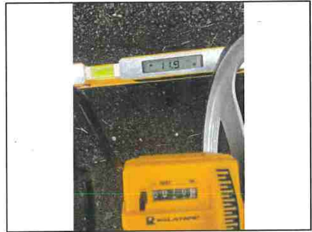
Photo #52 Private Access Rd Slope 11.9% Width 10'7"
