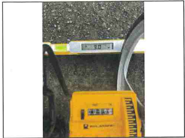
Photo #14 Private Access Rd Slope 9.0% Width 16'5"
