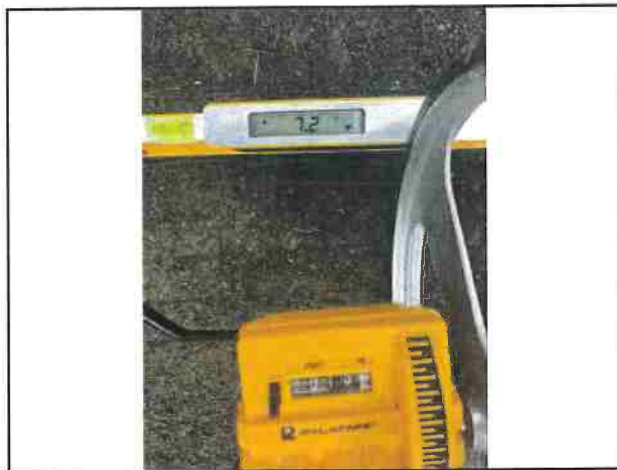
Photo #41 Private Access Rd Slope 7.2% Width 13'2"
