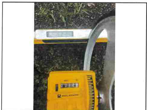
Photo #36 Private Access Rd Slope 16.2% Width 12'1"
