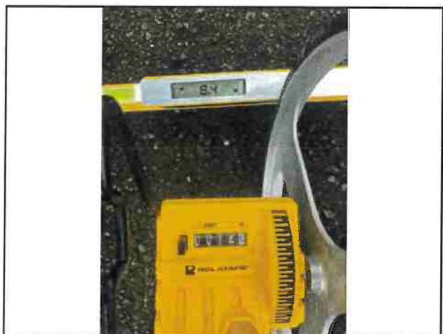
Photo #60 Private Access Rd Slope 8.4% Width 12'0"
