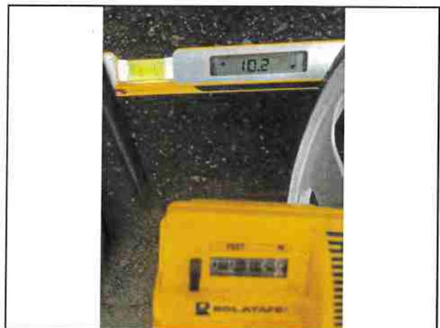
Photo #94 Private Access Rd Slope 10.2% Width 12'2"
