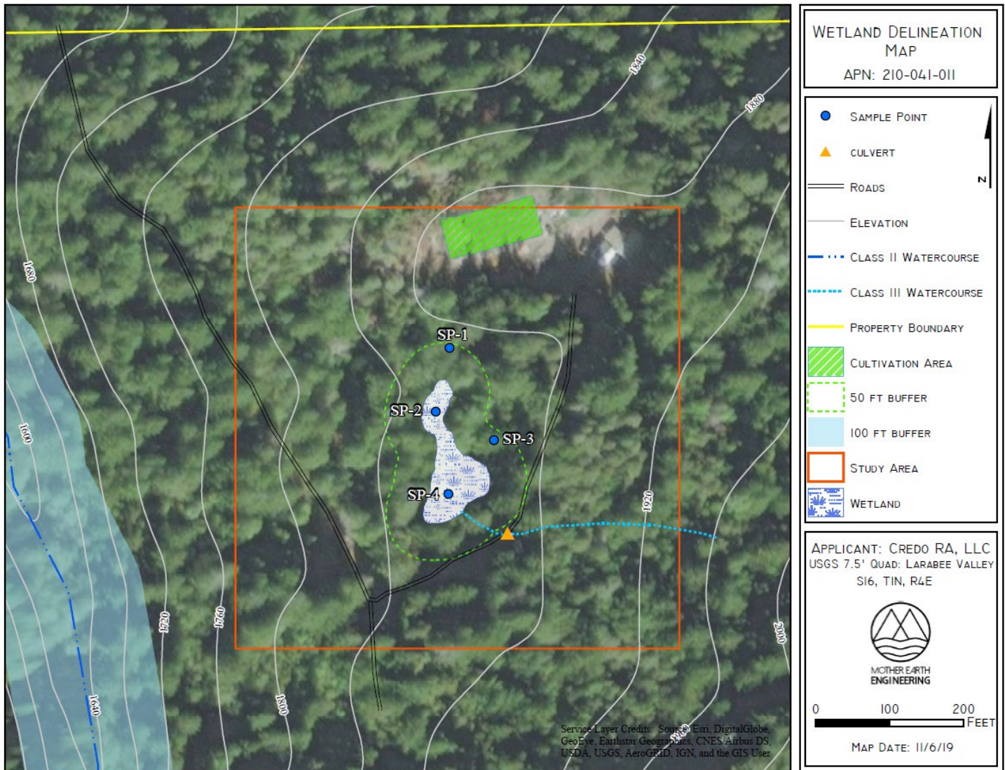
Figure 5. Map of wetland extent and boundaries within the study area. A 50 ft buffer designated around the wetland is outside cultivation activities.
